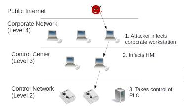
Fig. 6: Attacker using vertical movement to compromise PLC from the corporate network
