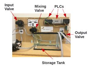
Fig. 2: Water Treatment Testbed
