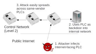
Fig. 5: Attacker using PLC for horizontal movement within the internal network
