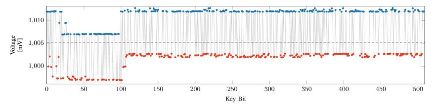
Fig. 13: Core voltage per measured instruction for each key bit offset in the fixed window length implementation of mbed TLS inside an SGX enclave on the Xeon E3-1275 v5. The blue marks represent 1 bits, while the red marks represent 0 bits. Using a threshold (dashed line), they can easily be distinguished.
